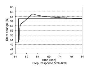
Figure 4 Response Characteristics of Normal PID Control
