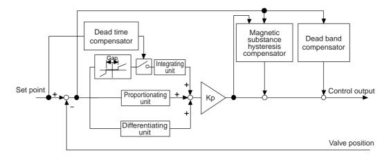
Figure 3 Block Diagram of PID Control with Nonlinearity Compensation
