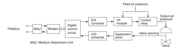
Figure 2 Block Diagram of YVP110
