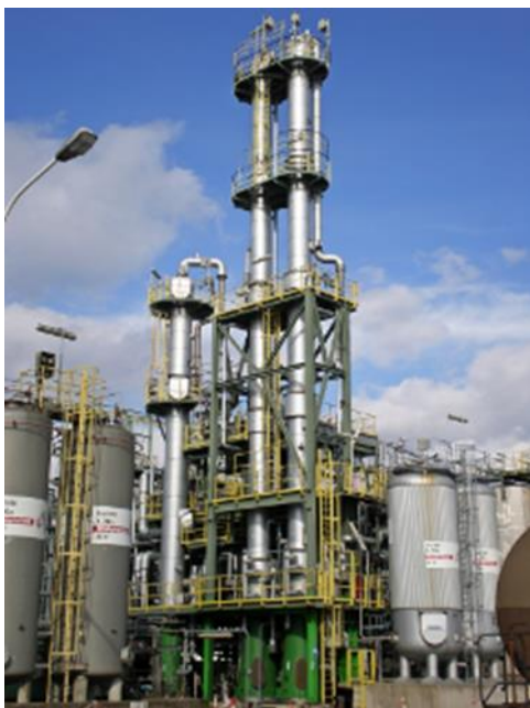
Fig. 1 Distillation columns for processing the THF-water mixture at ISP Marl
