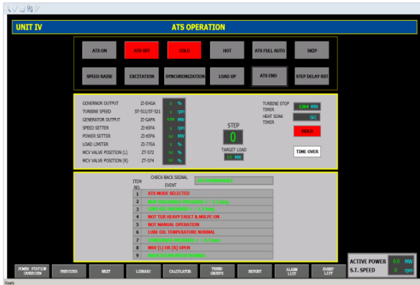
Automatic turbine startup window
