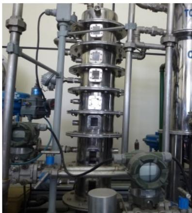
Transmitters measuring the pressure
