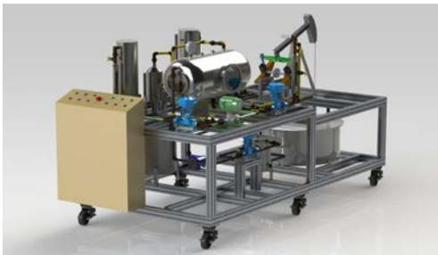
Micro pumping unit and three phase separator
