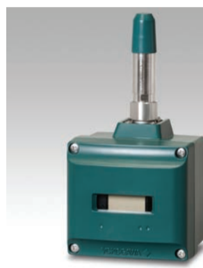
Fig.5. Yokogawa's multi-function wireless adaptor enables wired devices that transmit and receive digital on/off signals or receive 4-20 mA analogue signals to function as ISA100 Wireless™ field wireless devices
