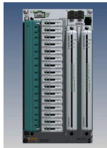
Fig.3. Yokogawa's N-IO (Network-IO) field I/O device for handling multiple types of I/O signals
